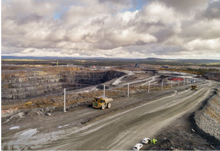
New Aitik electric trolley
