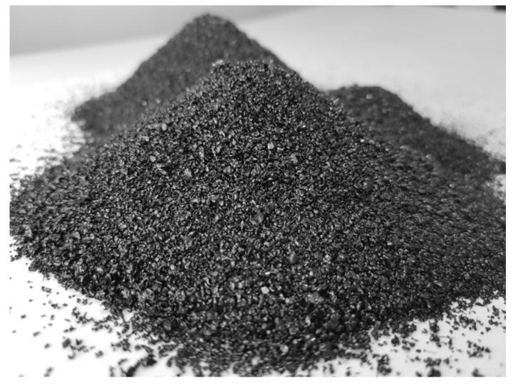
**IRON SAND** is a glassy iron silicate aggregate consisting of granulated slag, extracted as a by-product from Boliden Rönnskär's copper production.
