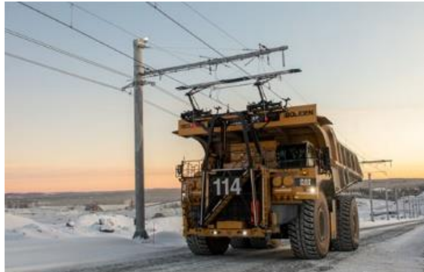
Present electric trolley at the Aitik mine
